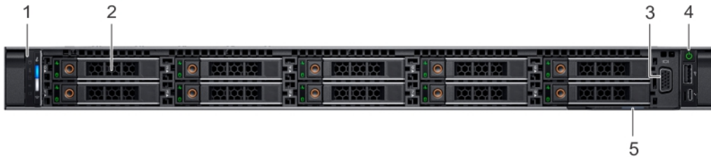
Figure 3. Front view of 10 x 2.5-inch drive system
