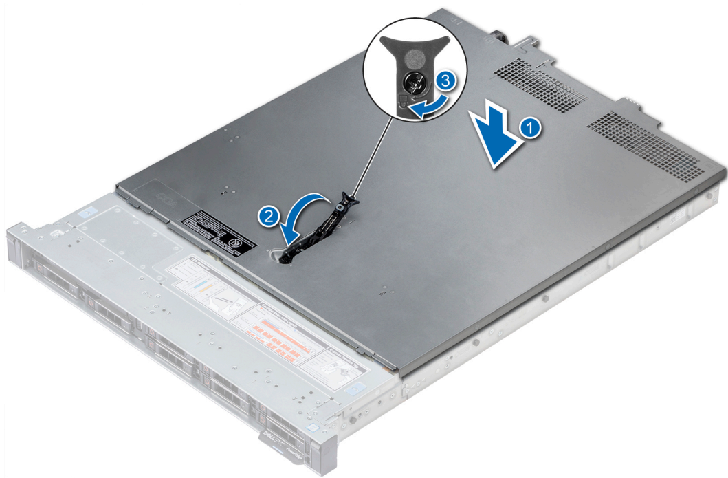
Figure 19. Installing the system cover
