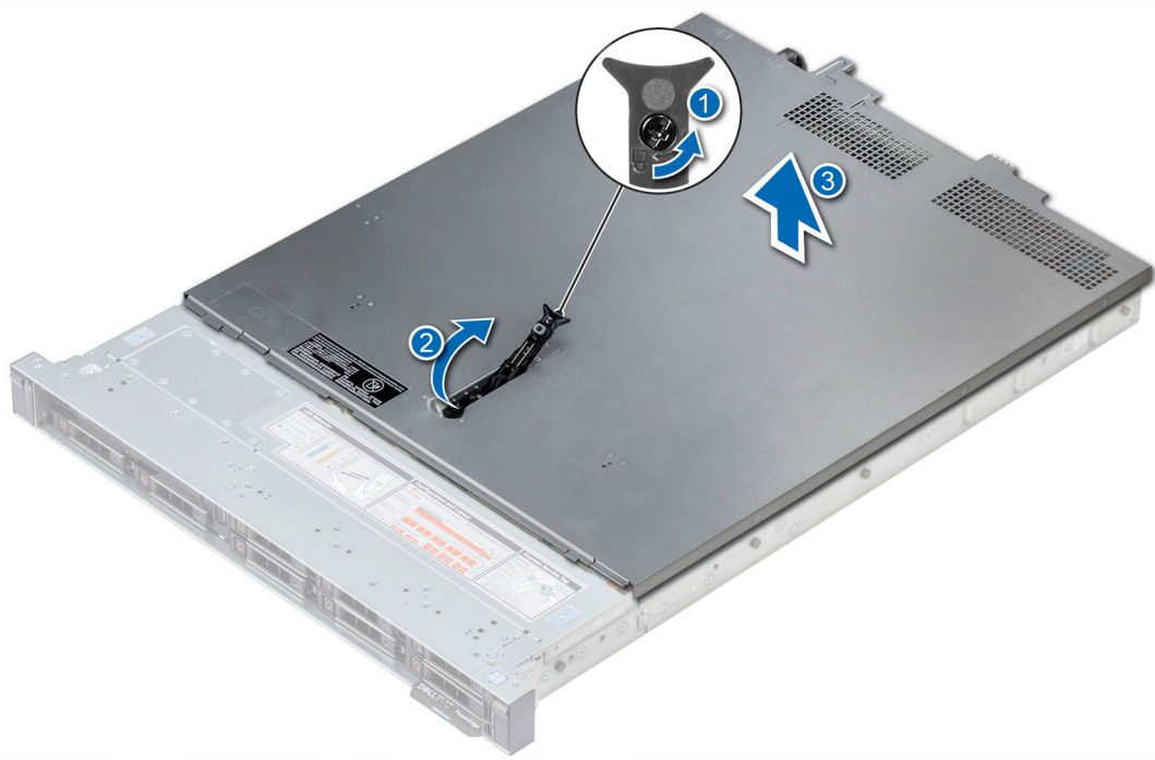
Figure 18. Removing the system cover
