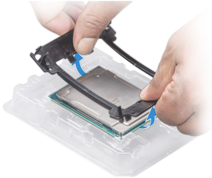
Figure 44. Removing the processor bracket
