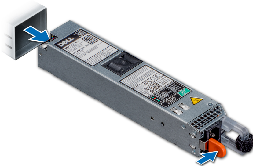
Figure 100. Removing a power supply unit
