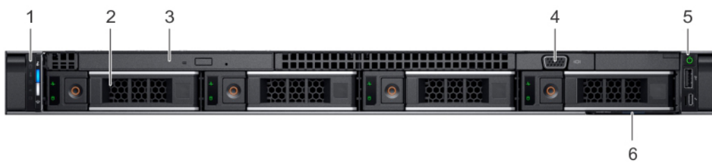
Figure 2. Front view of 4 x 3.5-inch drive system
