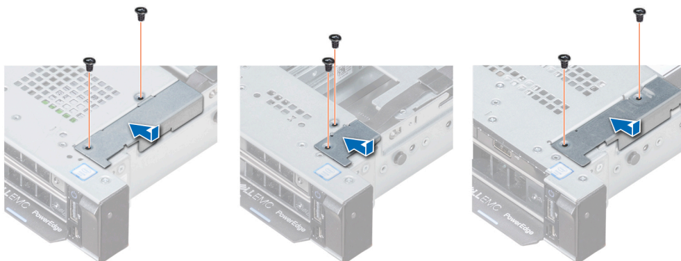
Figure 111. Installing the cable cover
