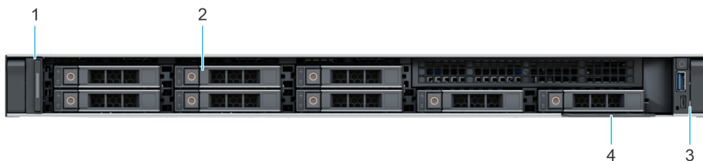
Figure 1. Front view of 8 x 2.5-inch drive system
