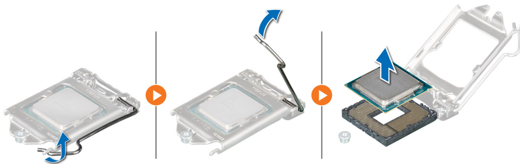
Figure 43. Removing the processor
