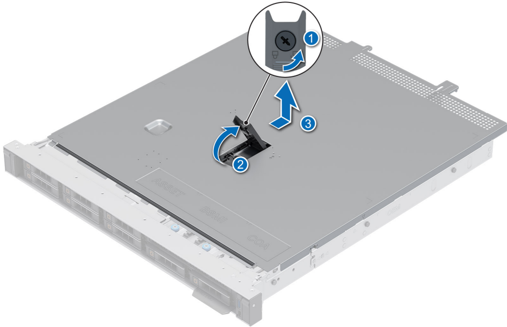
Figure 11. Removing the system cover
