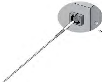
Figure 67. Cleaning a Recessed Ferrule
