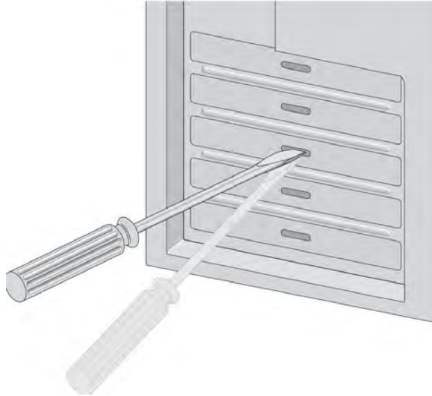
Figure 13. Removing the Faceplate From PCIe Slot
