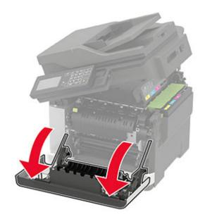
3 Open the fuser access door, and then remove the jammed paper.Note: Make sure that all paper fragments are removed.
