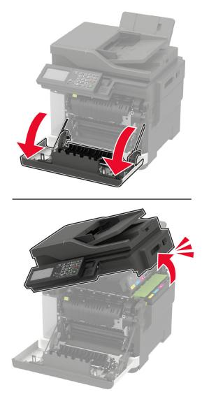
**2** Open the fuser access door, and then remove the jammed paper.
