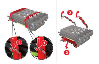
**Note:** If you are replacing the black imaging kit, then insert the magenta, cyan, and yellow developer units into the new imaging kit.
