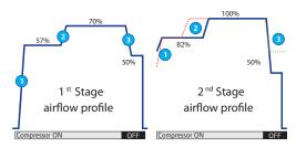
Direct Drive motor shall be variable speed type with constant airflow setting. Motor will be ECM (Electronically Commutated Motor) as standard preprogrammed with enhanced airflow capabilities.
