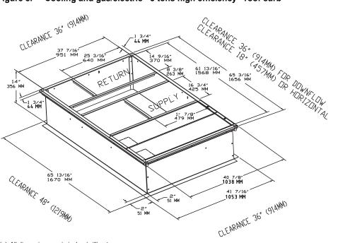
Figure 9. Cooling and gas/electric - 3 tons high efficiency - downflow duct connections - field fabricated<sup>(a)</sup>
