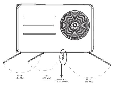
Figure 13. Gas/electric models - 3 tons high efficiency height of gas pipe required from inside base of unit to gas shut off assembly (factory provided) - Y\_C models only<sup>(a)</sup>
