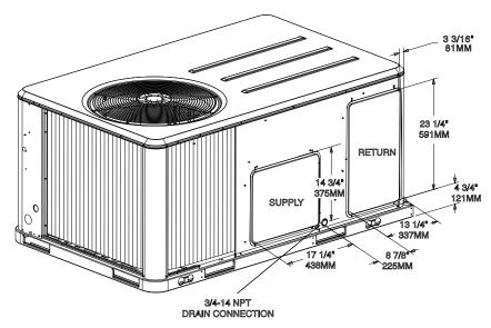
Figure 7. Cooling and gas/electric - 3 tons high efficiency, unit clearance and roof opening<sup>(a)</sup>
