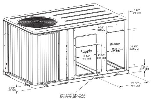
Figure 17. Cooling and gas/electric - 4-5 tons high efficiency - unit clearance and roof opening<sup>(a)</sup>
