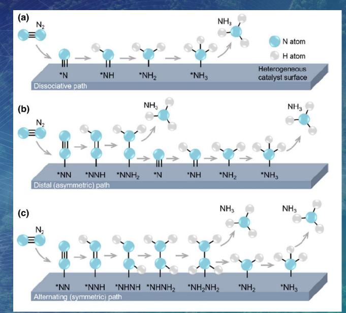
Nitrogen reduction pathways in heterogeneous CAT dissociative pathway where the N≡N bond is broken before hydrogenation. Association pathways that include B) distal or asymmetric hydrogenation and C) alternating or symmetrical hydrogenation.
