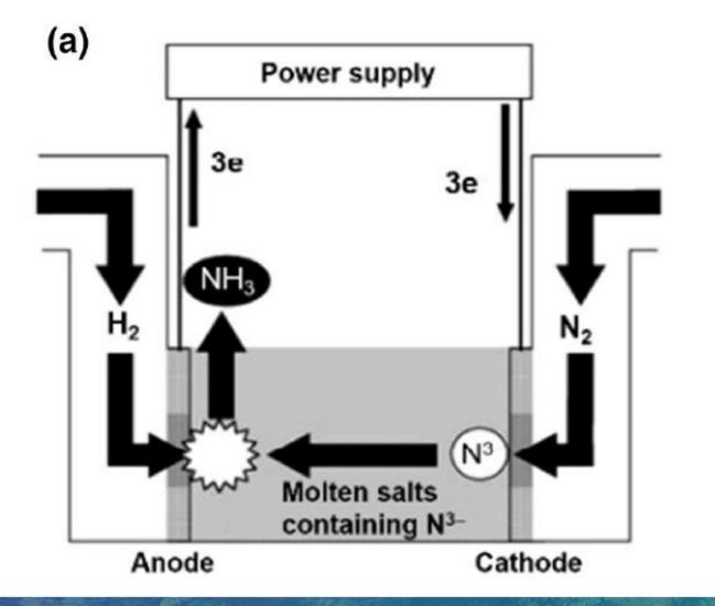
Electrochemical synthesis of NH3 in molten electrolytes. Scheme of the principle of electrolytic synthesis of NH<sub>3</sub> from N<sub>2</sub> and H<sub>2</sub> in molten salts of LiCl–KCl– CsCl containing N<sub>3</sub>–.
