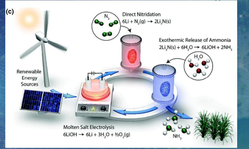
C) Scheme of a lithiummediated step-by-step cycle process for sustainable production of NH3 from N2 and H2O driven by renewable energy sources
