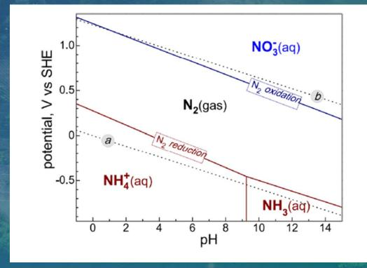
Partial Pourbaix diagram for the N2–H2O system. The red line represents the reduction of N2 to NH4 + or NH3, while the blue line denotes oxidation of N2 oxidation to NO3 –. Dashed lines a and b represent reduction of H2O to H2 and oxidation to O2, respectively.
