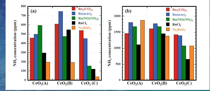
$NH_3$  synthesis activity of various 1 wt% Ru/CeO<sub>2</sub> catalysts prepared using the indi-cated catalyst and support precursors. a NH3 concentration in the effluent gas. b Maximum NH3 concentration. Catalyst weight: 0.2 g, flow rate: 80 mL/min (H2/N2 = 3), ambient pressure, 325 °C
