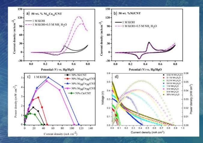
(a) The current density of 50 wt% Ni50Cu50/CNT; (b) The current density of 50 wt% Ni/CNT; (c) Comparison of power density between various catalysts for AOR; (d) The maximum power density for the ammonia fuel cell made with NiCu/C and single-phase perovskite oxide
