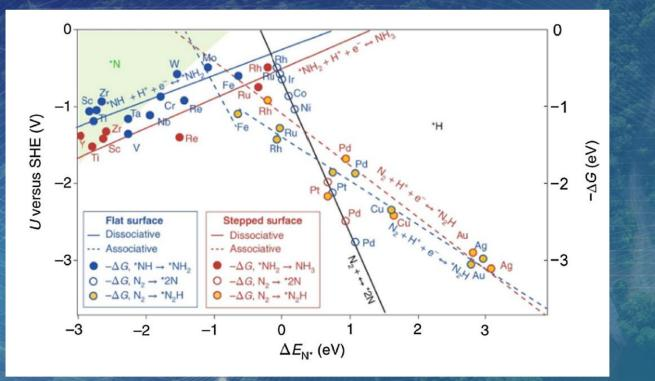
Combined volcano diagrams evaluating the onset potential (U) on different transition metals. Solid lines represent dissociative mechanisms and dashed lines represent associative mechanisms.
