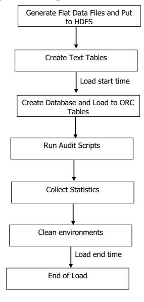
Figure 3.8: Block Diagram of Database Load Process
