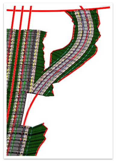
13. Before placing the asphalt template drop, we need to set a **point control** on the mainline corridor. Select the **Prop EOP - CTRL** feature definition (Linear >> Roadway >> Model Control - 2D Plan >> EOP), if not still selected.
