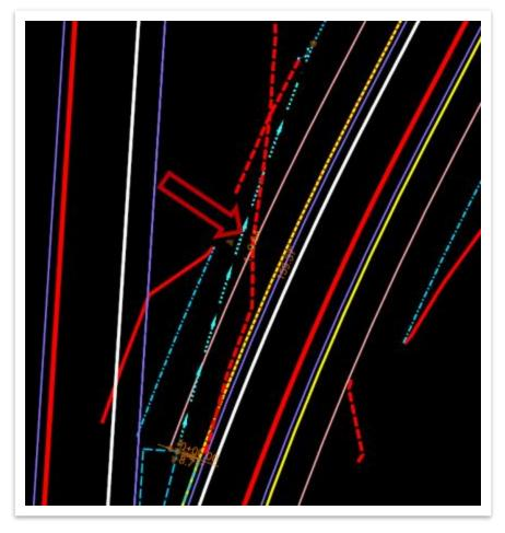
6. For both ditch lines placed, change the offset Slope to -16.67% in the properties of the horizontal line and then complex the ditch lines together. Once completed, open the profile of the complex line. Go ahead and complex the two profile lines and set the complex profile to active.
