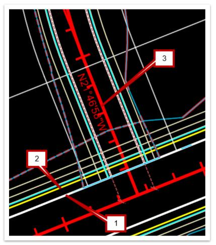
Make sure the placement looks correct by clicking on the control lines. In this exercise, there should be no need to reverse the direction of the reference lines. Right click to accept line directions. Next, select the Side Road corridor to clip and then right click to accept. Lastly, left click to accept the civil cell placement.
