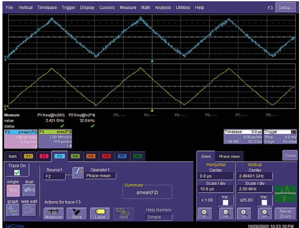
See multiple cycles of spread spectrum clocking.
