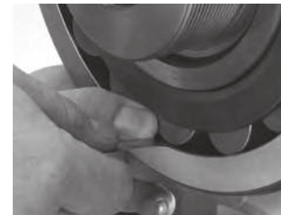
Fig. E-4. During mounting, the RIC should be checked at the unloaded roller.
