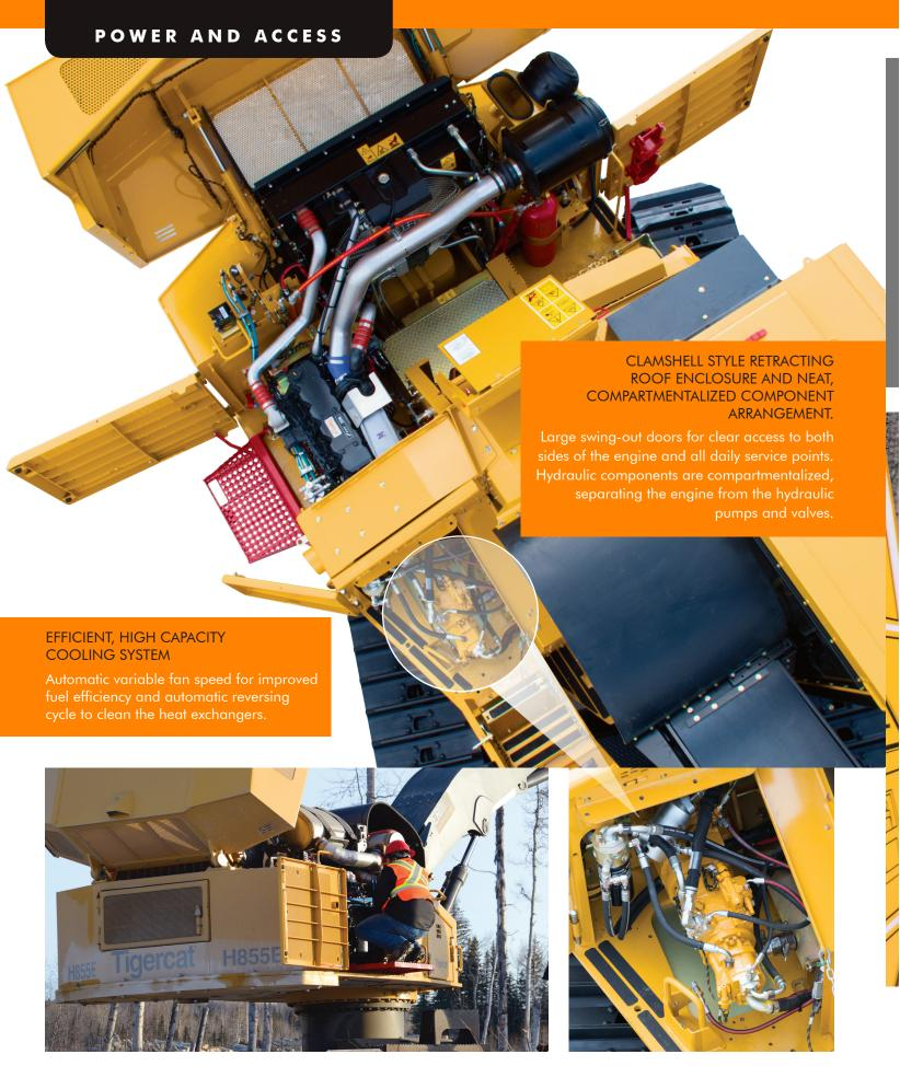
Swing-out door with service platform allowing quick and easy engine access.
