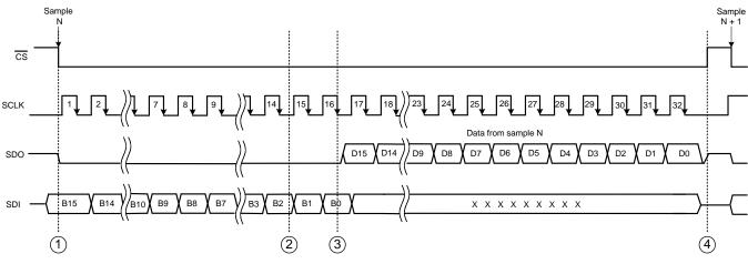
Figure 16. Device Operation Using the Serial Interface Timing Diagram
