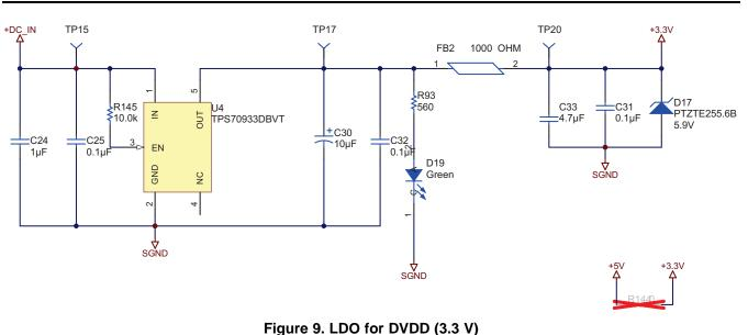
**NOTE:** The ADS8688 device can be configured to operate with single supply. Remove the components shown in Figure 9 and populate R144 to configure the ADC for 5-V operation.
