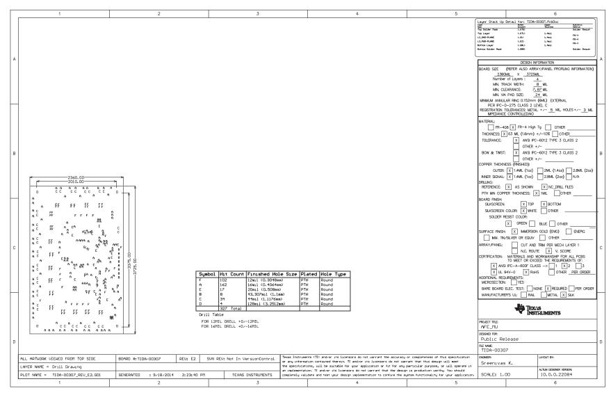
Figure 44. Fabrication Layer
