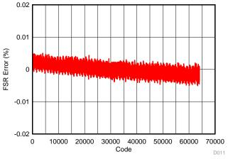
Figure 22. 0 to 5-V Range, Code versus FSR Error (%) After Calibration
