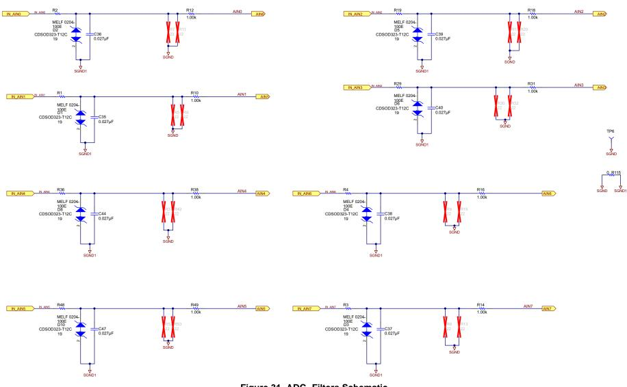
Figure 31. ADC<sub>1</sub> Filters Schematic
