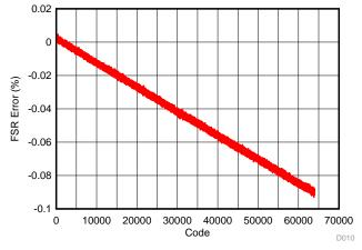
Figure 21. 0 to 5-V Range, Code versus FSR Error (%) Before Calibration
