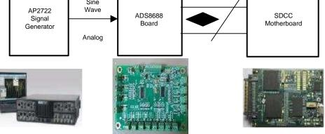
Figure 20. ADC Measurement Setup
