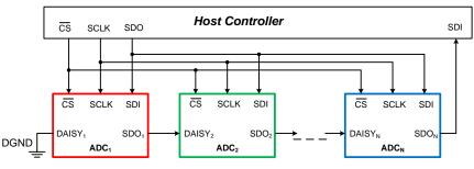
Figure 7. Daisy-Chain Diagram
