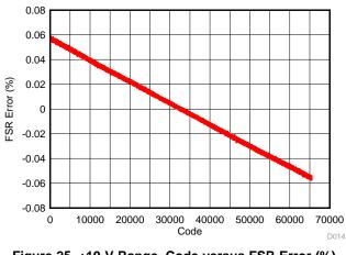
Figure 25. ±10-V Range, Code versus FSR Error (%) Before Calibration
