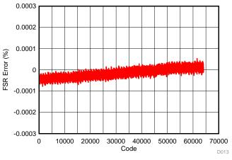
Figure 24. 0 to 10-V Range, Code versus FSR Error (%) After Calibration
