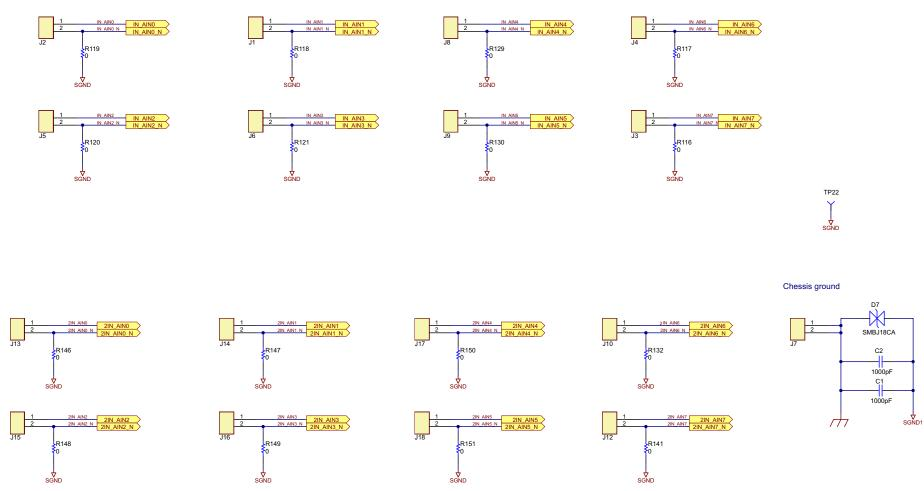
Figure 30. ADC<sub>1</sub> and ADC<sub>2</sub> Inputs Schematic
