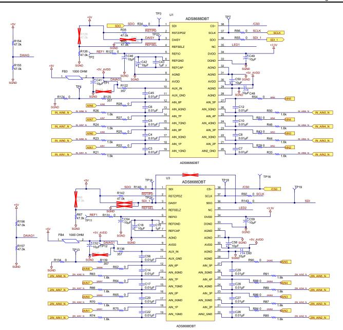
Figure 6. Two ADCs Connected in Daisy Chain Mode
