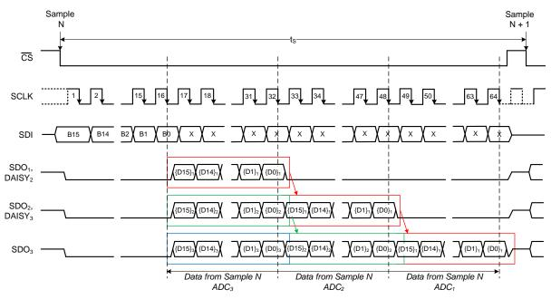
Figure 8. Timing Diagram for Devices Connected in Daisy-Chain Mode
