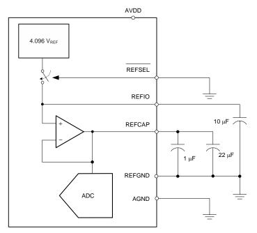
Figure 5. ADS8688 Connections for Using an Internal 4.096-V Reference
