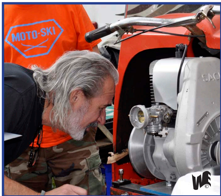
A potential buyer goes eye to eye with the carburetor on a Sachs motor as he inspects a snowmobile of interest.
