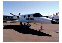
Powered by two jet engines and a rocket engine, the Rocketplane XP is a heavily modified Learjet 25 capable of reaching sub-orbital space. Image credit: Incredible Adventures/Rocketplane Limited, Inc.
