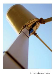
of a satellite feedhorn. we are peering down the brace. The feedhorn selects the polarity of the waves helps to attenuate Space Products and Services | 3.0 adjacent channels and transponders, Space products and services rely upon space and from other communications infrastructure, are in the space environment, satellites at nearby or operate in it or through it, and include
