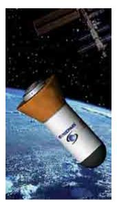
The largest spacecraft planned for Spacehab's Apex family is its 400 series, capable of carrying payloads of up to 12,300 kilograms. *Image credit: Spacehab*
