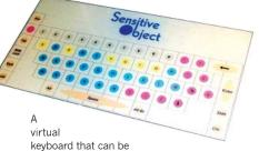
Applied to a variety of materials is being developed with technology previously used on accelerometers in the inertial postioning system onboard Ariane launches. Vibration sensors are mounted on the product to detect which area is touched. It is easy to maintain and has no moving parts. *Image credit: Sensitive Object*
