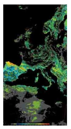
Realtime Normalized Difference Vegetation Index (NDVI) data from a NOAA Advanced Very High Resolution Radiometer (AVHRR). NDVI is a quantity that measures greenness and vigor of vegetation. *Image credit: RSGB, University of Bern, and NOAA*  or region. Exhibit 2q breaks down the number of communications satellites attributed to each country or organization.
