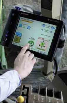
One of the 2006 inductees to the Space Foundation's Space Technology Hall of Fame,<sup>®</sup> Novariant AutoFarm's systems link farm vehicles with GPS tracking, enabling accurate handsfree navigation of fields. This increases efficiency and allows crews to work longer—even in the dark. *Image credit: AutoFarm*
