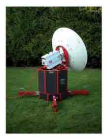
VSAT dish in remote setting readied for transmissions. Image credit: TC Communications Very Small Aperture Terminal Services: VSAT networks transmit data, voice, and video among an unlimited number of geographically dispersed sites. VSAT networks use satellites operating in C-, Ku-, or Ka-bands. Examples of VSAT data services include linking field offices to headquarters, client transactions such as credit-card verifications, and ATM transactions.
