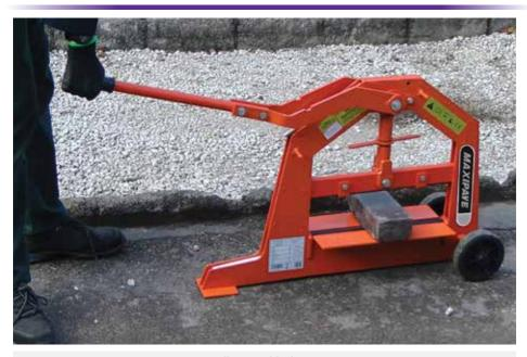
Small paving block cutter
