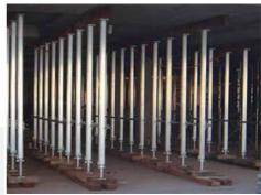
Heavy duty Aluminium Super props / Multi props
