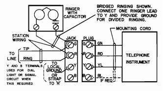
Fig. 2-1 PORTABLE INSTALLATION WIRING
