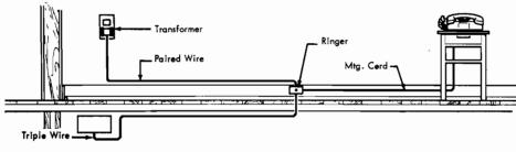
Fig. 3-1 DIAL LIGHT TRANSFORMER WIRING
