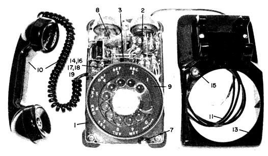
Fig. 1 TOP VIEW - HOUSING REMOVED
