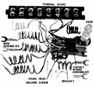
Fig. 2-1 TYPICAL TURN AND PUSH KEY
