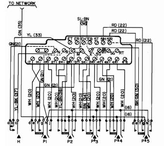
All PICK-UP keys interlocked to allow only one to be in operated position at any time. Operation and release of (non-locking) HOLD key releases any operated PICK-UP key. Interlocking may be disabled on any or all of keys PS3, PS4 and PS5 to convert them to non-locking interphone signalling keys. c) Type 589(B)740
