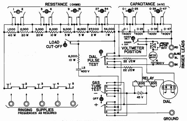
Fig. 3-1 RINGER TEST SET - CIRCUIT DIAGRAM
