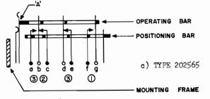
Insertion of .025" shim between spring and operating bar at "A" with cradle hook depressed must not operate any contacts point
