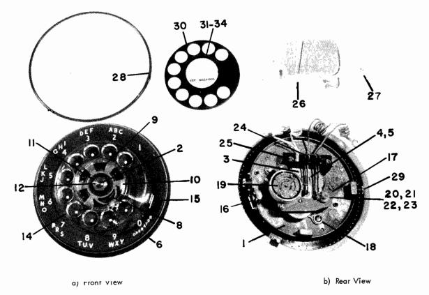
Fig. 1 IDENTIFICATION OF DIAL PARTS
