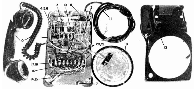
Fig. 1 TOP VIEW - HOUSING REMOVED
