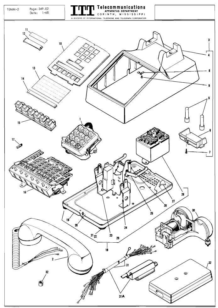
Figure 2. K-1564 and K-2564 Key Telephones, Exploded view.
