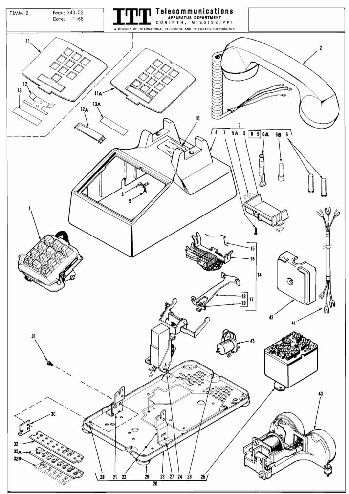
Figure 2. Single line "TEL-TOUCH" desk telephones, exploded view.
