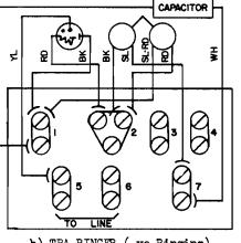
b) TBA RINGER (-ve Ringing) Fig. 2 RINGER WIRING (AS SHIPPED)
