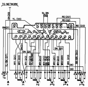
All PICK-UP keys interlocked to allow only one to be in operated position at any time. Operation and release of (non-locking) HOLD key releases any operated PICK-UP key. Interlocking may be disabled on any or all of keys PS3, PS4 and PS5 to convert them to non-locking interphone signalling keys.
