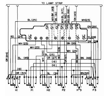
Keys interlocked in pairs. Operation of HOLD key releases interlocked PICK-UP key and vice versa. All PICK-UP keys interlocked to allow only one to be in operated position at any time. Any operated hold keys are automatically released when the handset is replaced in the cradle. Interlocking may be disabled on key HS3 to convert it to a nonlocking interphone signalling key.
