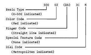
2.2 The availability of colors and the possible combinations of ringers, special features and dials, are noted in the descriptive sub-section for each type of telephone. The sub-section index for the example shown is 500/30.
