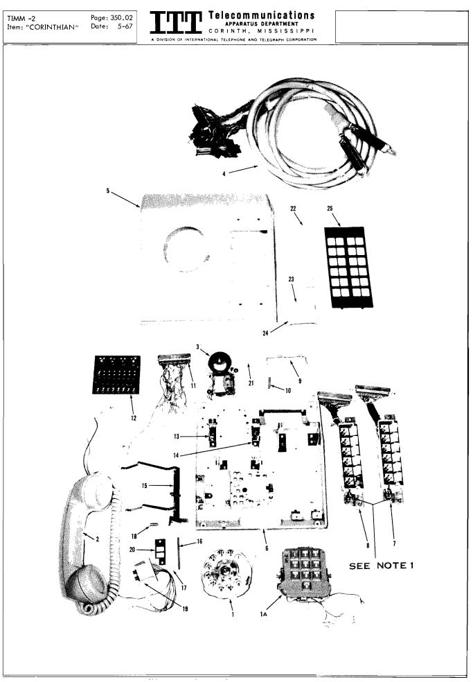
Figure 2. "CORINTHIAN" Telephone, Exploded View
