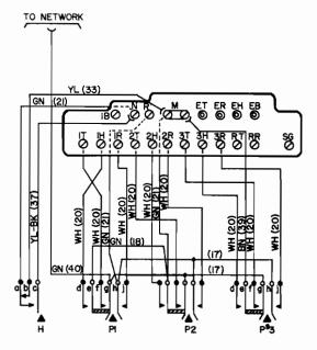
All PICK-UP keys interlocked to allow only one to be in operated position at any time. Operation and release of (non-locking) HOLD key releases any operated PICK-UP key. Interlocking may be disabled on key PS3 to convert it to a non-locking interphone signalling key.
