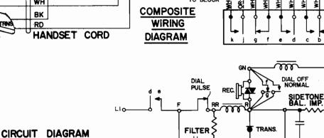
Connect yellow mounting cord lead as shown by dashed lines. Mounting cord connections shown for ring party. For tip party reverse red and green cord conductors on ringer terminal board and use
