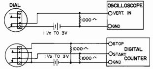
Note: Circuit for stop and gate signals may have to be modified for some types of digital counter.
