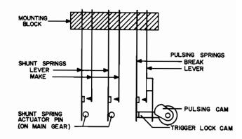
Fig. 3 CONTACT ARRANGEMENT
