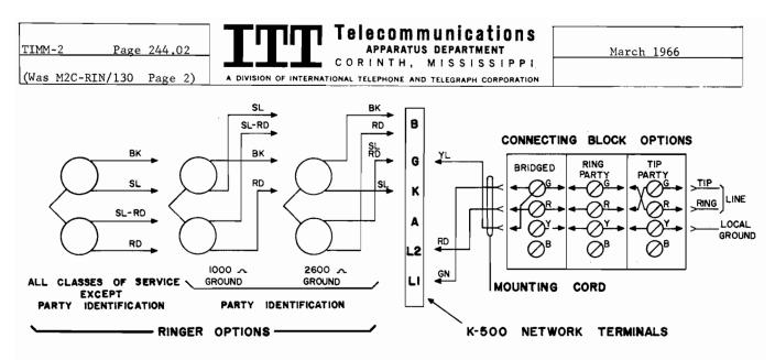
Fig. 2 TYPICAL WIRING DIAGRAMS
