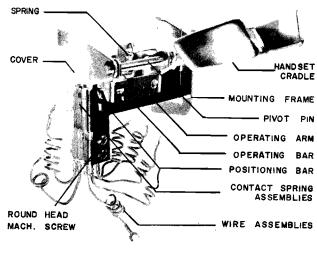
Fig. 2-1 TYPICAL HOOK SWITCH
