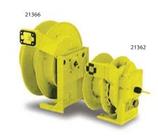
IMPORTANT NOTE: Retractable Reel Model 21362 will store and operate w/a maximum of 40' #2 Str., 1/0 Str. and2/0 Str. grounding cable only. Retractable Reel Model 21366 will store and operate w/a maximum of 65' 1/0 Str., 60' 2/0 Str. and 50' 4/0 Str. To order Reel Model 21366 w/cable and clamp factory installed, specify
