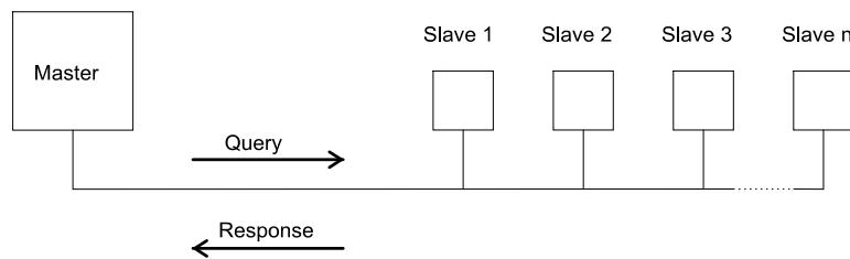
In the MODBUS™ Protocol the master can address individual slaves, or, using a special “Broadcast” address, can initiate a broadcast message to all slaves. The Integra, INT-2270, INT-2170 digital power quality meter does not support the broadcast address.
