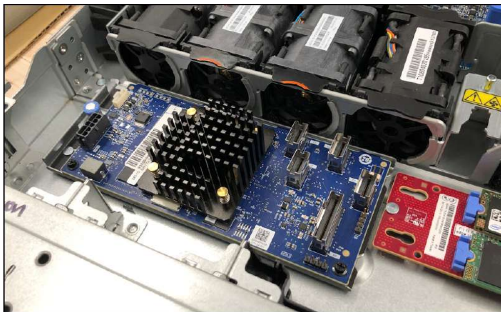
Figure 11. ThinkSystem RAID 940-16i Internal Adapter (front drive backplane removed to show the adapter)
