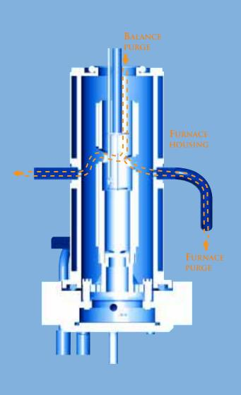
• Furnace Our custom designed furnace is the second key element of a Q Series<sup>™</sup> TGA. It features low mass, rugged heater windings, and proprietary heater control technology. *Benefits:* Rapid, accurate and precise temperature programming over a wide range, plus optimized use of advanced techniques such as Hi-Res<sup>™</sup> TGA and Modulated TGA<sup>™</sup>. Our reliable, long-life furnaces also increase the value of your investment
