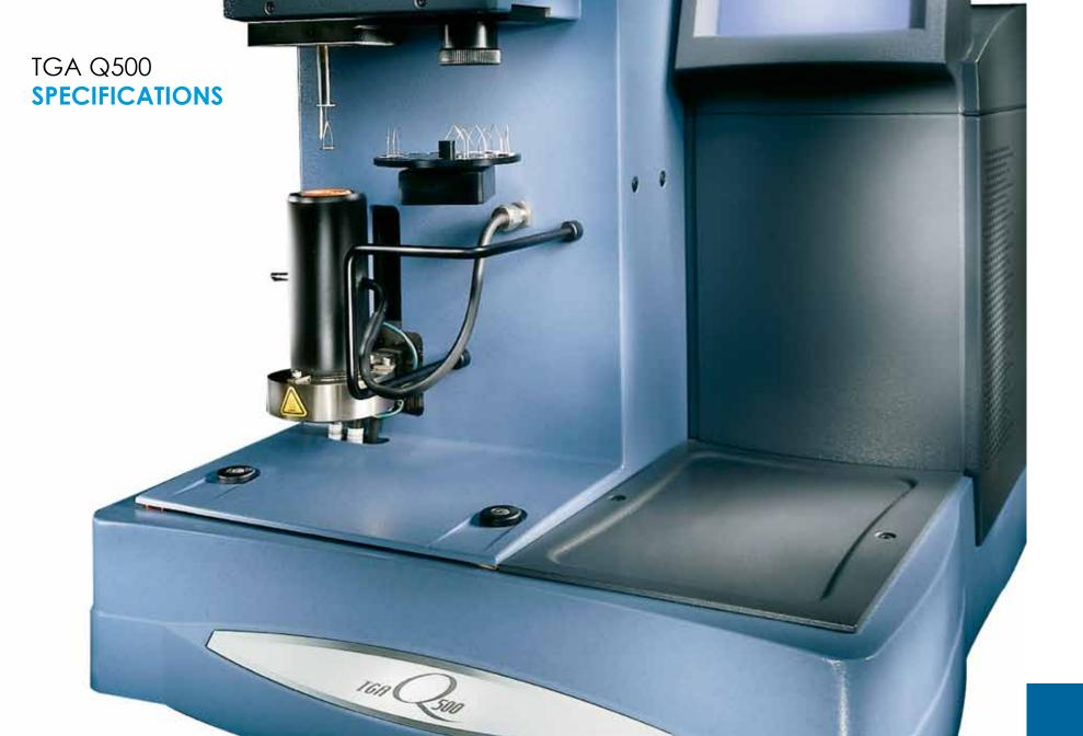
The Q500 is the world's best-selling, research-grade thermogravimetric analyzer. Its field-proven performance arises from a responsive low-mass furnace, ultrasensitive thermobalance, and efficient horizontal purge gas system with mass flow control. Its convenience, expandability and powerful, results-oriented software make the Q500 ideal for the multi-user laboratory where a wide variety of TGA applications are conducted, and where future expansion of analytical work is anticipated.
