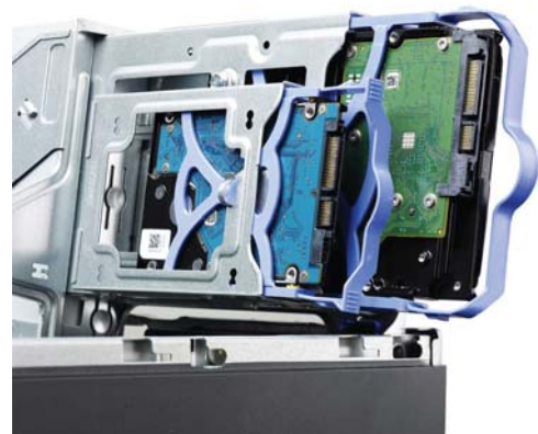
Optional 2.5" bay on Lenovo ThinkCentre M93/M93p Small Pro * Come with optional 2.5" 2nd HDD
