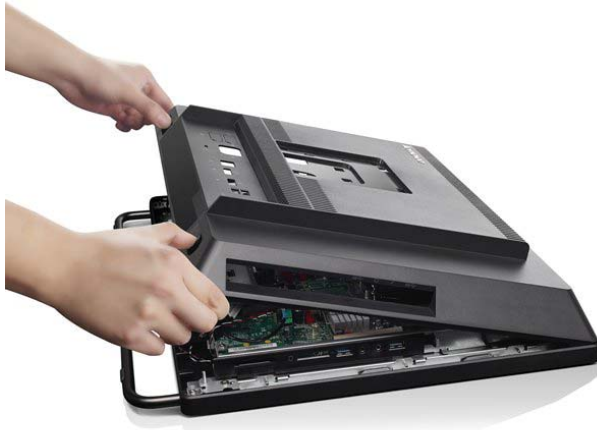
Toolless Back Cover Removal
