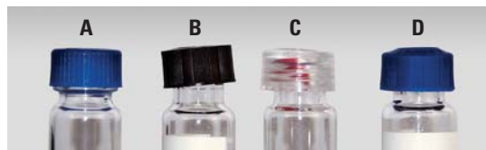
Examples of vial and closure misalignment/deformation. (A) SureStop vial self aligning cap; (B) generic vial, cap tilt; (C) generic vial, septum dislodged; and (D) generic vial, deformed top.
