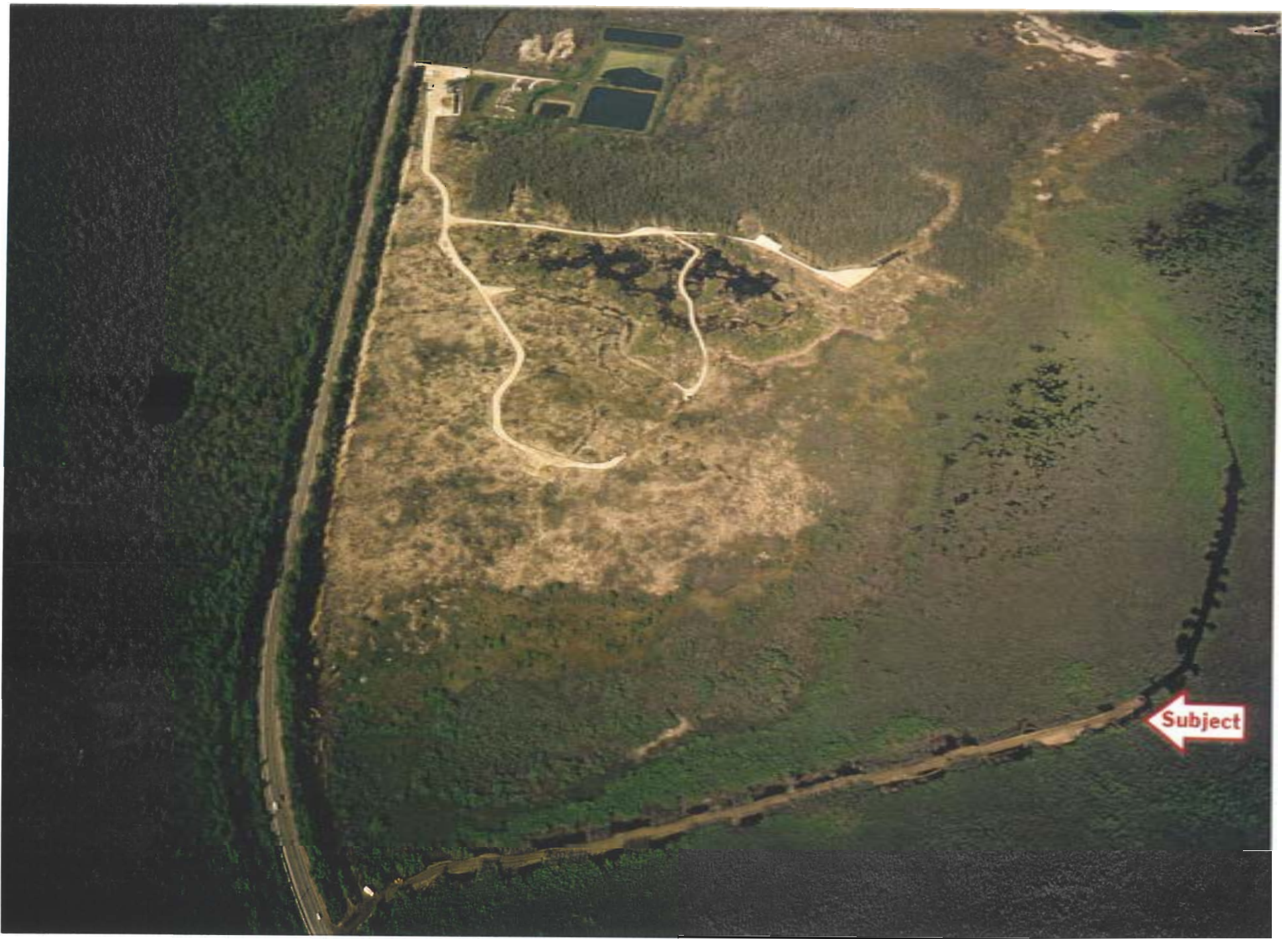
SEPTEMBER 1997 - PHASE I HYDROLOGIC RESTORATION AT LITTLE PINE ISLAND - DRAINAGE CANALS ARE FILLED TO RESTORE SHEET FLOW
