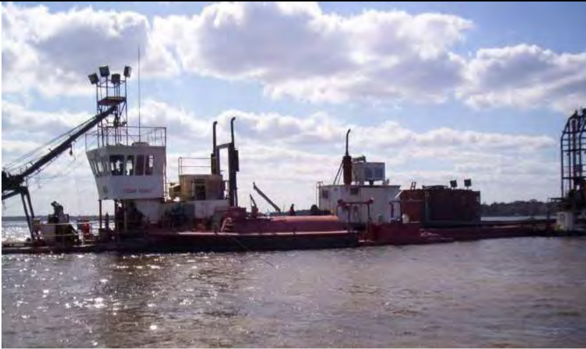
View of the barge used to hydraulically dredge the inorganic sediments accumulated within the bottom grades of Lake Panasoffkee.
