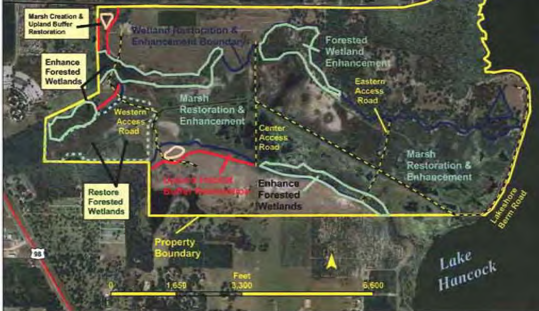
Figure E - SW 66 - Circle B Bar Reserve Post-Construction Wetland Restoration & Enhancement Areas
