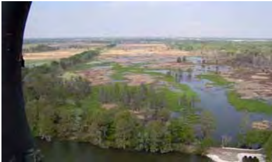
View of the former northeast bahia pasture, with the tree-lined eastern segment of the Banana Creek Canal spoil material evident to the left. This photo was taken after the north rim ditch was backfilled and hydrology restored, but prior to supplemental planting in the open water area. The new outfall to Lake Hancock includes culverts installed within the lakeshore berm (lower right).
