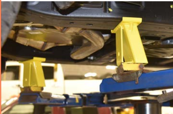
Front Adapters have 7" Wide Lifting Area
