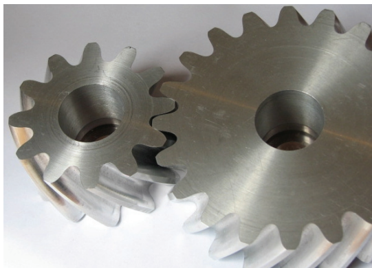
Fig. 17. A pair of the UPT gears; m_n=5\text{ mm} ; z_1=12 , z_2=20
