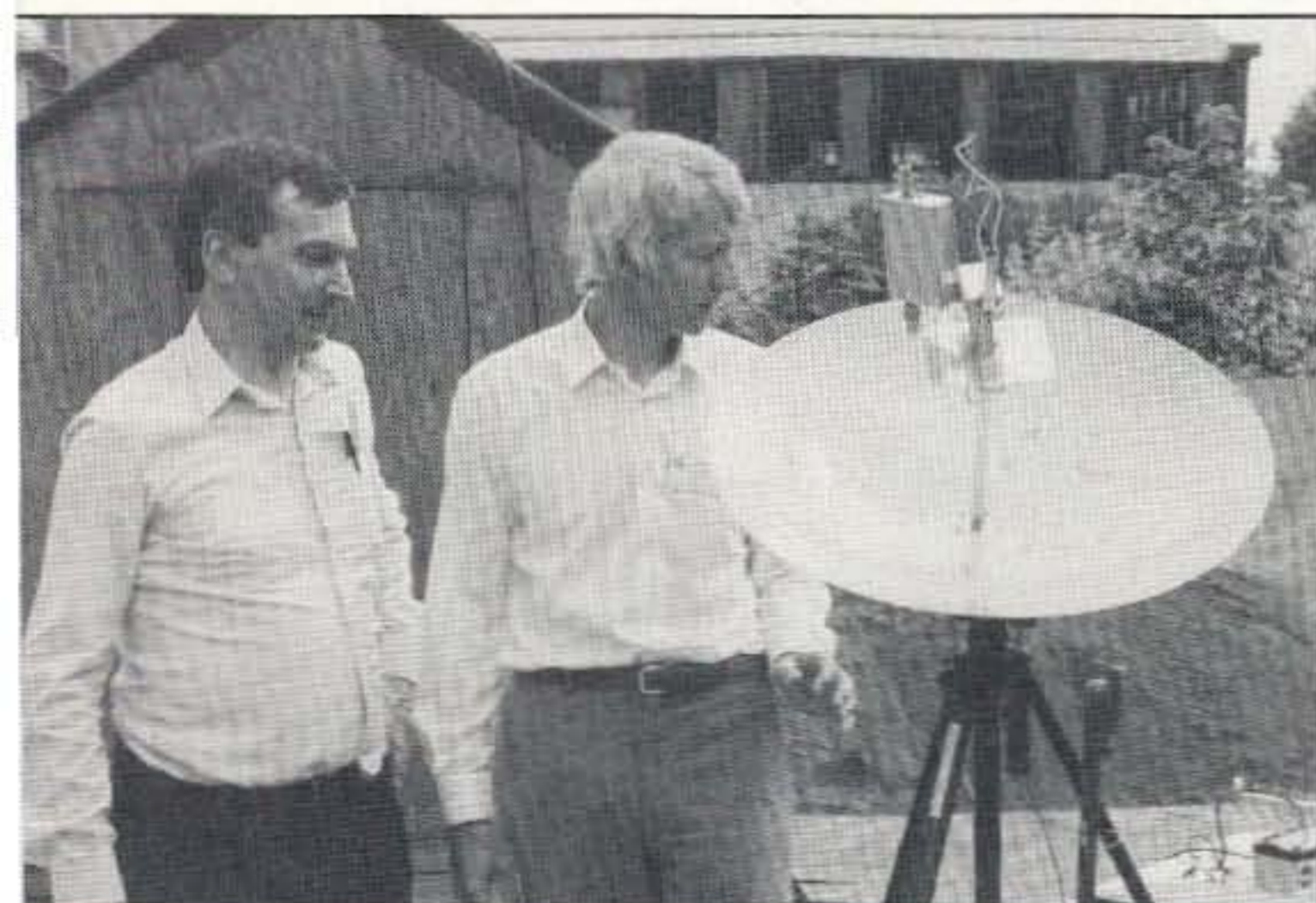
Photo C. Freddy De Guchteneire ON6UG and James Miller G3RUH demonstrated small dish for 2.4 GHz amateur satellite reception at the AMSAT-UK meeting. (W5IU photo.)
