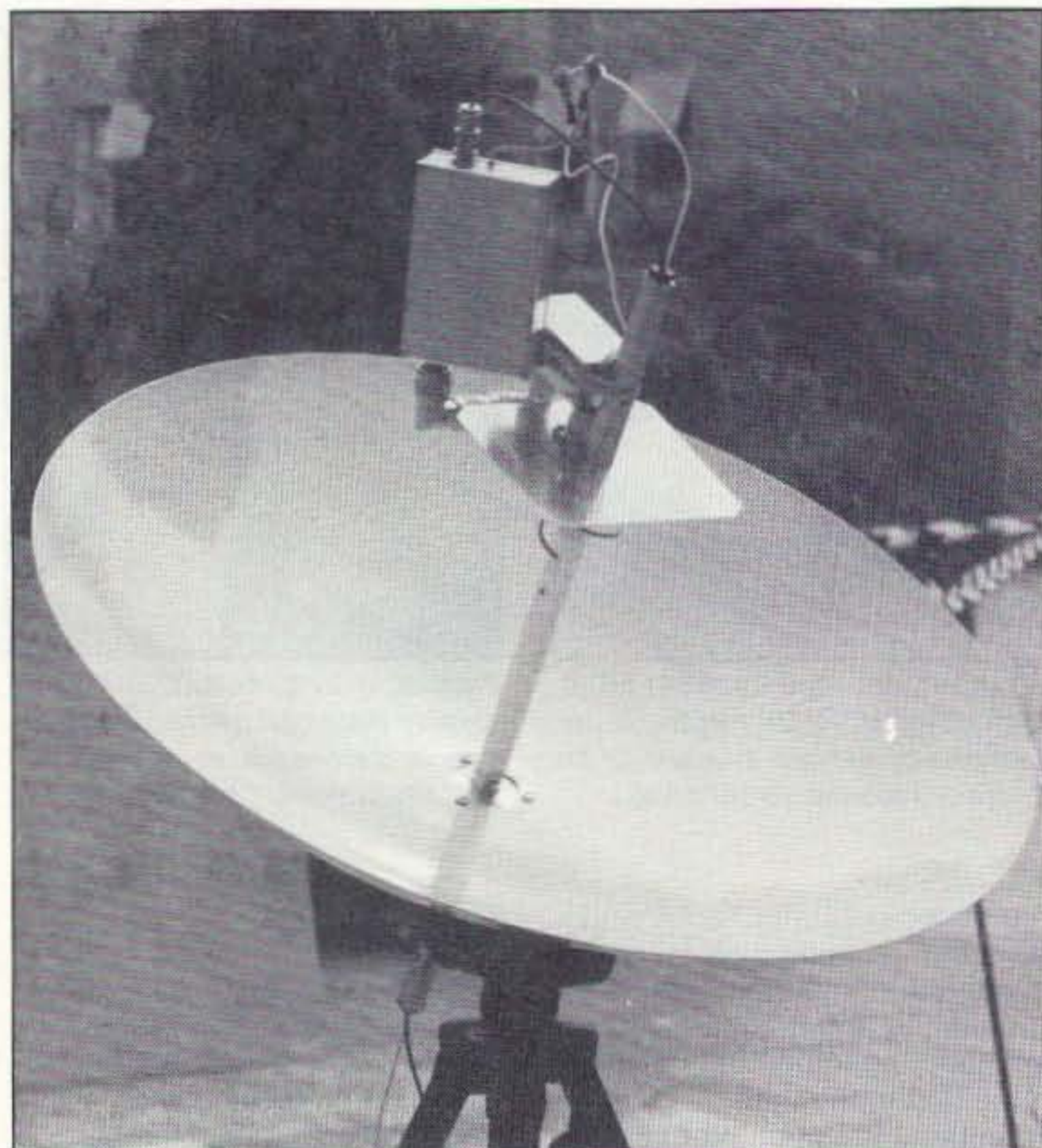
Photo D. A close-up of the G3RUH Mode "S" receive system. (W5IU photo.)
