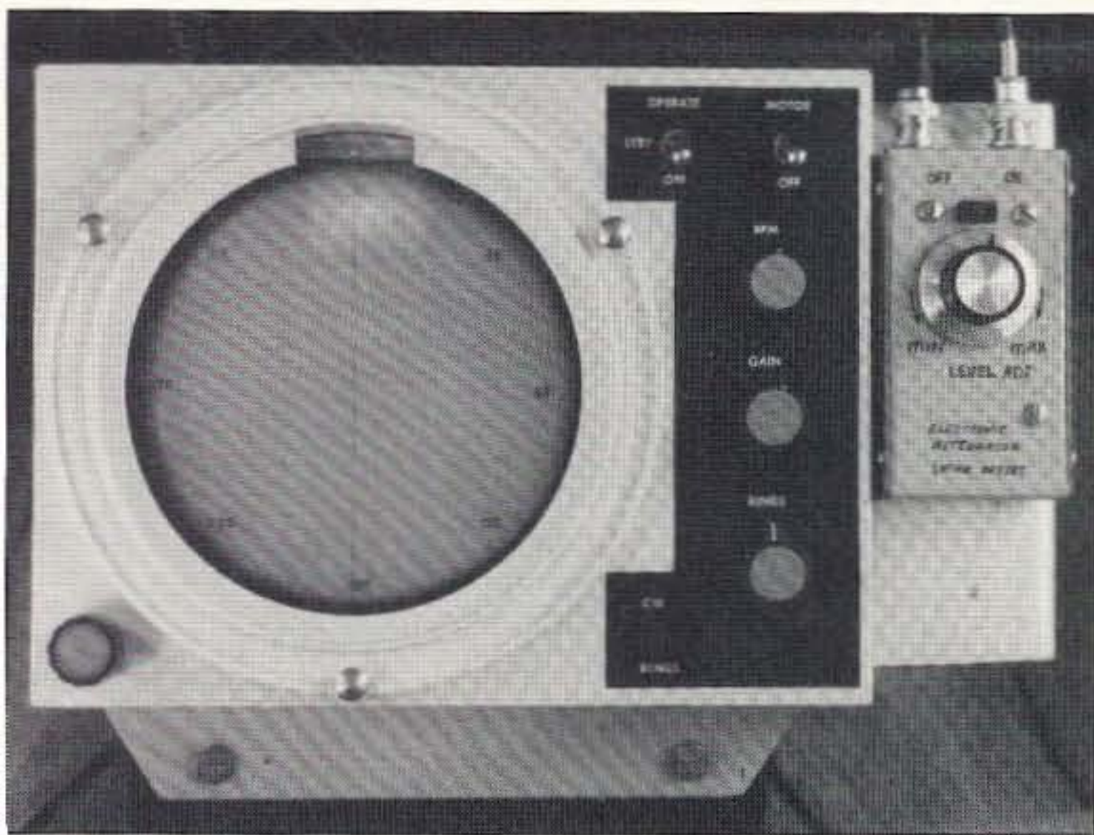
Photo B. The RADAD display unit mounts on the floor hump. Tom made a new front panel and mounted the RF attenuator box on a bracket for easy access.
