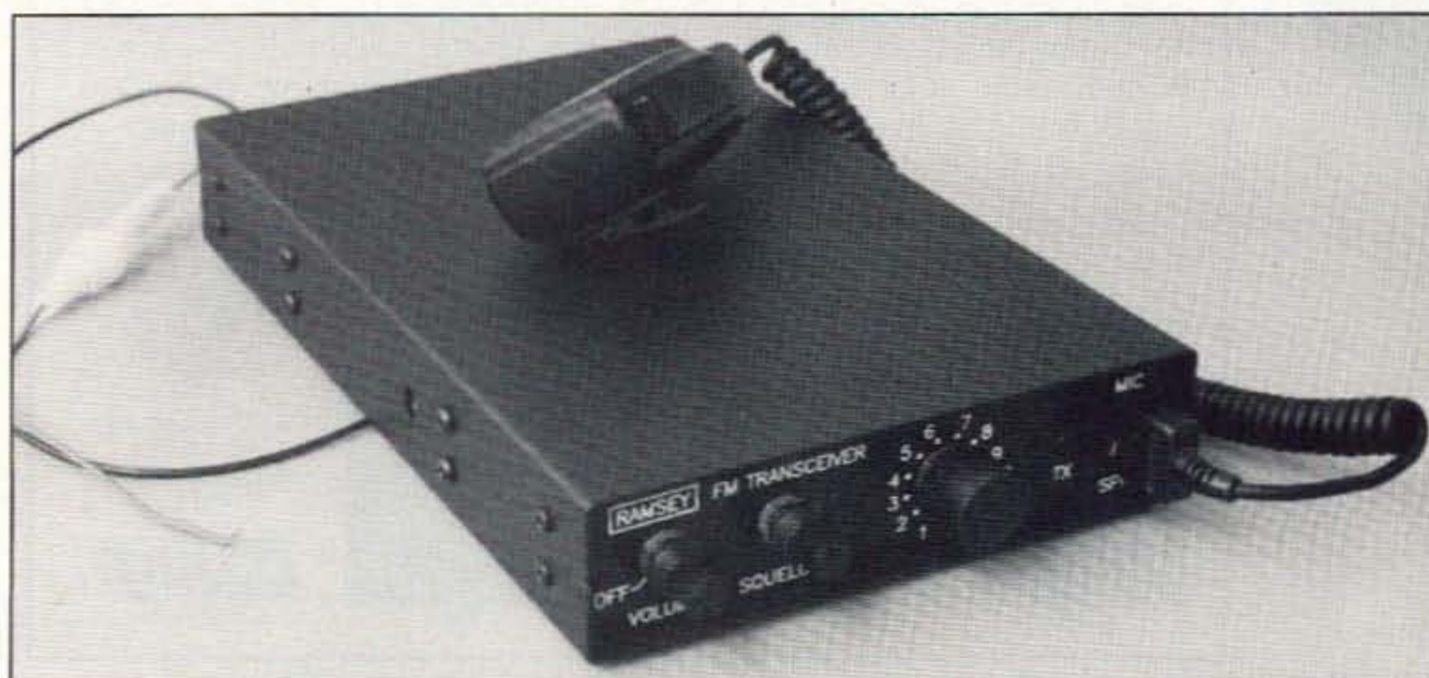
Photo A. The Ramsey FX-146 2m FM transceiver kit.
