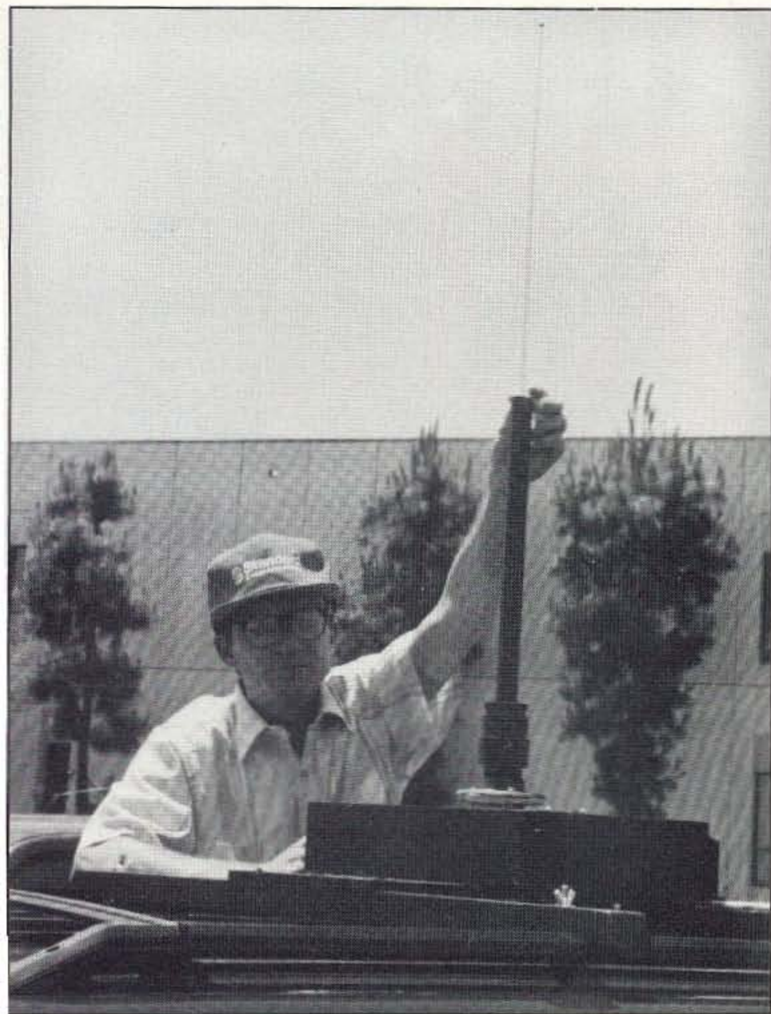
Photo D. Marine radar technician Tom King KA6SOX has taken off the yagi frame with parasitic elements and is holding the top of the driven element whip.
