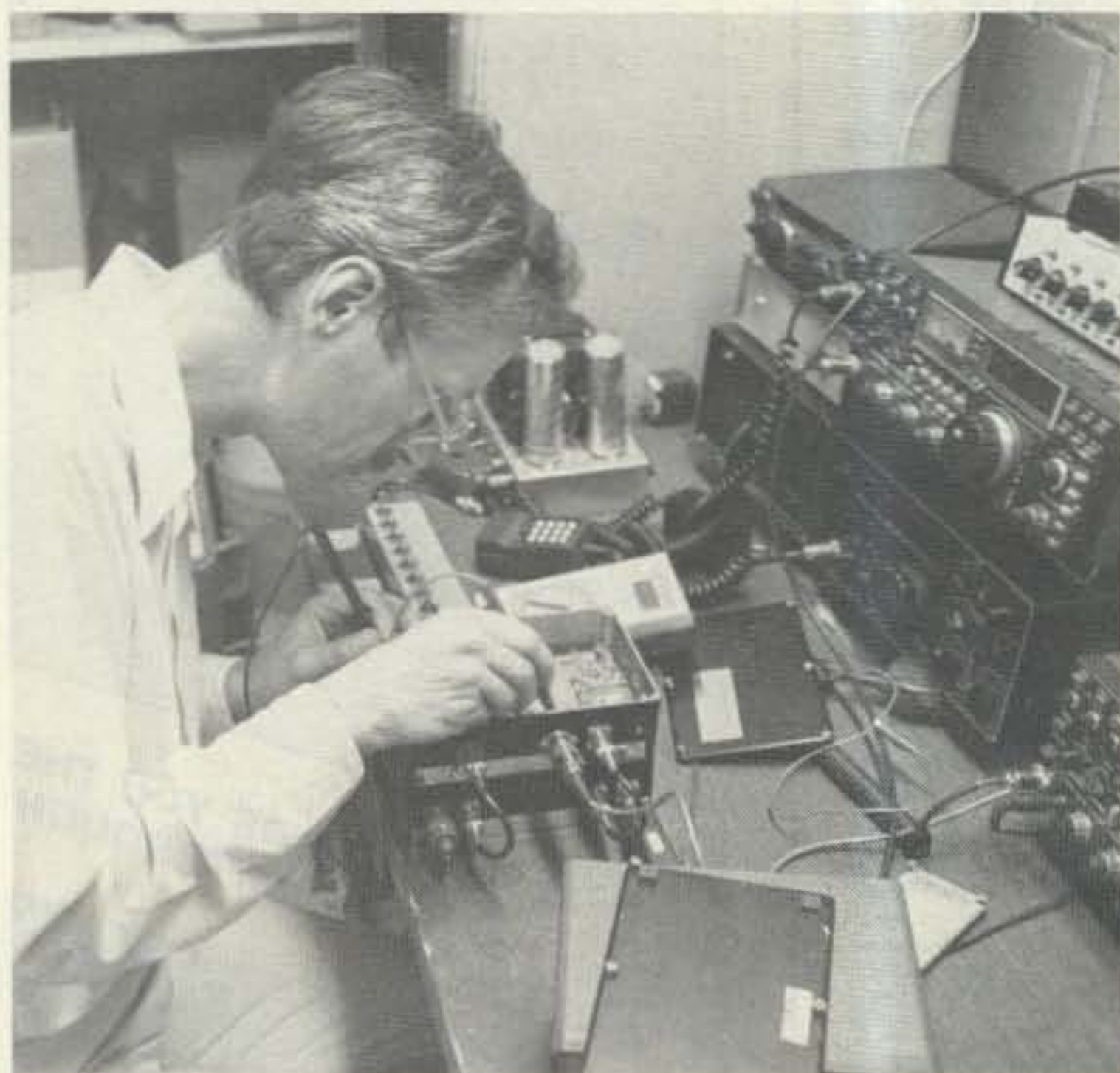
Hans VE3CRU fixing a sick 1296 Microwave Module.
