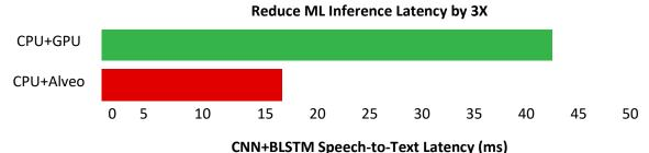
CPU+GPU: Nvidia P4 + Xeon CPU E5-2690 v4 @2.60GHz (56 Cores)
