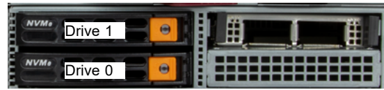
Logical drive numbers with jumper settings as shown on previous page.
