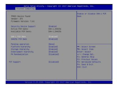
Disable "PH Randomization" and "TXT Support" only. Using the arrow keys, select each option, press the <Enter> key to select Disabled, and press the <Enter> key again. Press the <Esc> key to bring you back to the "Advanced" tab options. Use the arrow keys to toggle to the "Save & Exit" tab.
