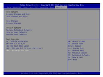
After Enabling TXT Support in the BIOS, you will need to run TXT in the UEFI shell. In the Command line at the bottom of the page, type "getsec64\_v2.0.11.efi -I sen -a" and press the <Enter> key. TXT support is now enabled.
