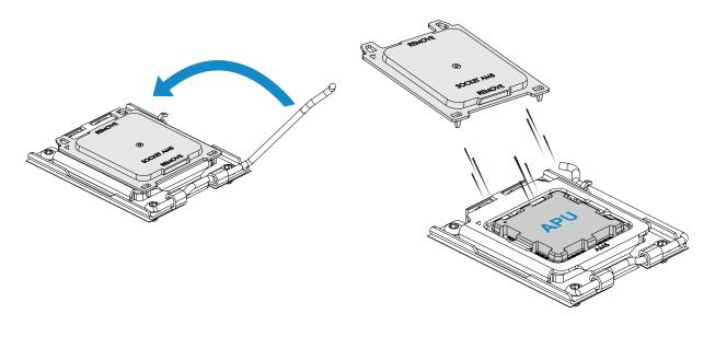
5. When finished, the socket force frame will secure the processor.
