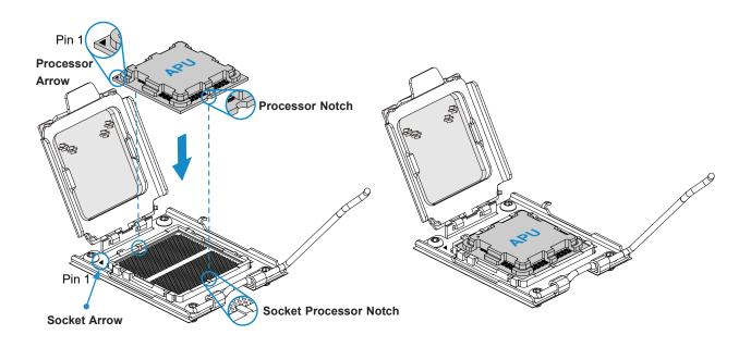
3. With the processor in the socket, lower the socket force frame.
