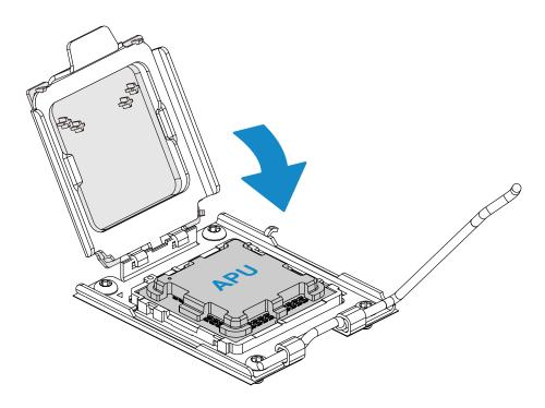
4. Reattach the lever arm onto the right side of the socket. The outer plastic cover will pop out when the lever arm is reattached.
