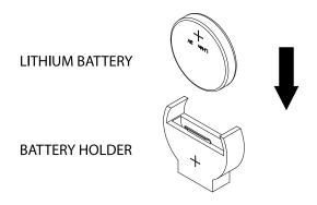
Figure 3-1. Battery Installation
