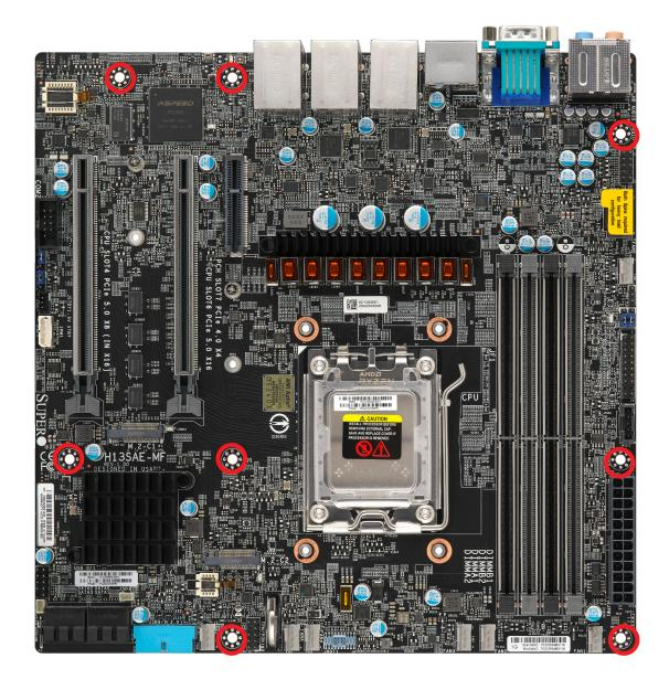
Figure 2-1. Motherboard Mounting Holes
