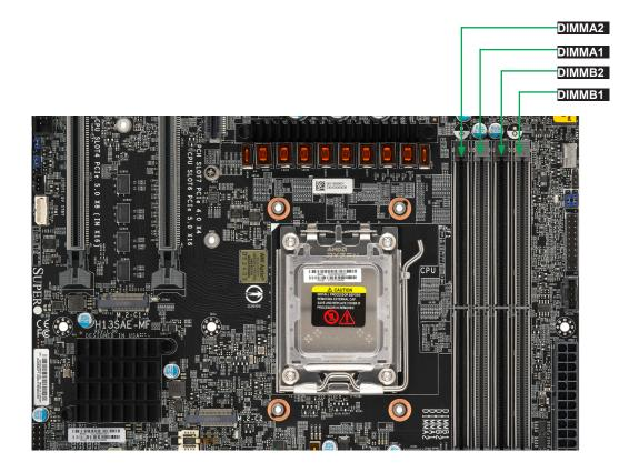
Figure 2-2. DIMM Numbering
