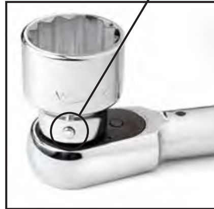
Socket-Lok® button positively locks the socket and drive tool together, providing positive retention and quick disassembly.
