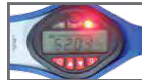
The red LED illuminates 4% beyond target torque, indicating fastener was overtorqued. Rapid "alarm" buzzer sounds.
