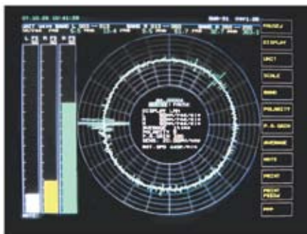
▲ Example in which nm/rad is selected as the unit of waviness
