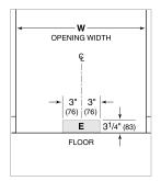
**IMPORTANT NOTE:** Adjacent countertops must be at least 35 7/8" for flush installation to top of unit.
