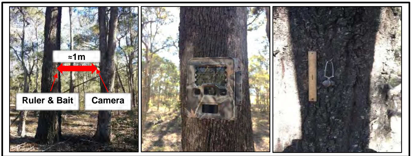
Figure 2: Remote camera trap and bait station used to detect squirrel glider presence.
