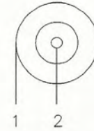
Figure 3-14 BNC Sockets, Female
