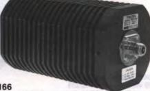
150 Watts- model 8166 Termaline® Load Resistor Power Rating 150W continuous Frequency Range & VSWR 1.1 max. dc to 1000MHz, 1.2 max. 1000 to 2500MHz Ambient Temperature Range -40°C to +45°C Connector QC Type (Female N normally supplied) Load Coolant Dry. Convection air cooled **Operation Position** Any Finish Semi-Gloss black enamel Nominal Size incl. conn. 731/64" x 4" sq. (190 x 102mm) Weight 96 oz. (2.7kg)
