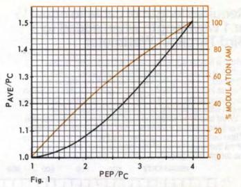
Correlation of PEAK-ENVELOPE-POWER (PEP), CAR-RIER POWER ( $P_c$ ), AVERAGE HEATING POWER ( $P_{AVE}$ ) and % MODULATION of AM signals of Table A, B or C below.
