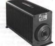
Specifications 600 Watts—model 8401 Power Rating 600W continuous Frequency Range & VSWR 1.1 max. dc to 1GHz, 1.2 max. 1 to 2.8GHz, 1.3 max. 2.8 to 3GHz Ambient Temperature Range -40°C to +45°C Connector QC Type (Female N normally supplied) Load Coolant 0.7 gal. (2.65 liters) Refined mineral oil Operating Position Horizontal only
