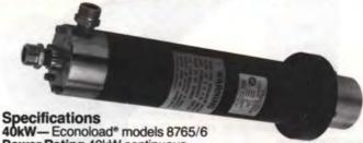
Power Rating 40kW continuous Frequency Range & VSWR 1.1 max. 1KHz to 900MHz (dc for continuity checks) Water Temperature Range +5°C to +60°C Water Flow Rate 8 to 10 gals./min. (30.3 to 37.9 liters/min.) Connector 8765 31/8" EIA FI, 8766 31/8" Unfl. Waterlines 1/2" FPT or 3/4" hose Load Coolant Potable water Operating Position Any Finish Semi-Gloss black enamel
