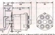
MOUNTING DIMENSIONS 7/32" (6mm) MTG HOLES FOR THREE 10-32 SCREWS SPACED AT 120° ON 11/4" (32mm) RADIUS
