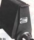
Specifications 1.5kW- series 8860 Power Rating 1500W continuous Frequency Range & VSWR 1.1 max. dc to 1000MHz, 1.25 max. 1000 to 2000MHz Ambient Temperature Range -40°C to +45°C Load Coolant 1.5 gal. (5.68 liters) Silicone Oil Operating Position Horizontal only Finish Light Navy grey baked enamel (MIL-E-15090)
