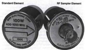
Coupler Elements: For RF signal observation on a scope, for spectrum analysis or for frequency counting and control, use Model 4274-025 wide range RF Sampler Element. This non-directional coupler delivers an unrectified signal at about -50dB ±2dB from 25-1000MHz tapering down to -66dB at 2MHz. Main line power should not exceed 500W.
