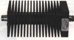
Tenuline® Attenuator Power Range 100W continuous Frequency Range dc to 1000MHz Ambient Temperature Range -40°C to +45°C Connectors QC Type (Female N normally supplied) Coolant Dry. Convection air cooled Finish Semi-Gloss black enamel Nominal Size incl. conn. 723/32" x 23/4" sq. (196 x 70mm) Weight 44 oz. (1.25kg)
