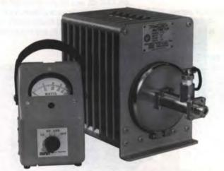
Specifications model 6732A **Power Rating 250W** Power Scales 10/50/250W Frequency Range & VSWR 1.1 max. 25-1000MHz Accuracy ±5% of full scale 25-512MHz, ±10% 512-1000MHz Connector QC Type (Female N normally supplied) Load Coolant 0.35 gal. (1.3 liters) Silicone Oil Finish Light Navy grey baked enamel (MIL-E-15090) Nominal Size Load 12%" x 8½" x 55%" (321 x 216 x 151mm); Meter 5%" x 3%" x 35%" (149 x 92 x 100mm) Weight 16 lbs. (7.2kg)
