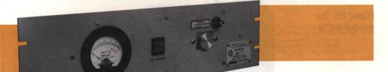
Model 4410P Panel-Mounted Wattmeter is electrically equivalent to the portable model 4411. It has a side door for battery replacement, a Universal Instrument-type AC connector and 150/230V rear selector switch, and fits into 51/4" space of standard 19" racks. RF Quick-Change Connectors can be changed without dismounting the 4110P from its rack.
