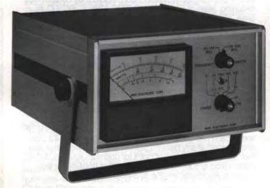
Specifications **Thruline Directional Wattmeter** model 4370 Power Ranges FWD 10, 25, 100, 500W; RFL 1, 2.5, 10, 50W Frequency Ranges 25-175MHz; 175-520MHz Insertion VSWR with N conn. 1.1 max. Accuracy ±5% of full scale Connectors QC type (Female N normally supplied) Finish Dark blue enamel and brushed aluminum Nominal Size 11" x 919/32" x 57/32" (277 x 244 x 133mm) Weight 71/4 lbs. (3.3kg)
