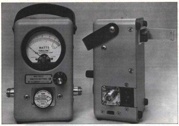
AC-powered models are equipped with a Universal instrumentation-type AC connector and an external 115/230V selector switch. Batteries are easily accessible through a batterycompartment door.
