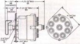
two-circuit, reversing switch model 72-R
