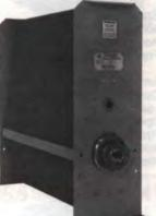
Specifications 5kW— series 8921 Power Rating 5000W continuous Frequency Range & VSWR 1.15 max. dc to 1000MHz Ambient Temperature Range -40°C to +45°C Load Coolant 6% gals. (25.3 liters) Silicone Oil Operating Position Horizontal only Finish Libtt Naw gray baked ename! (MIL =E-15090)
