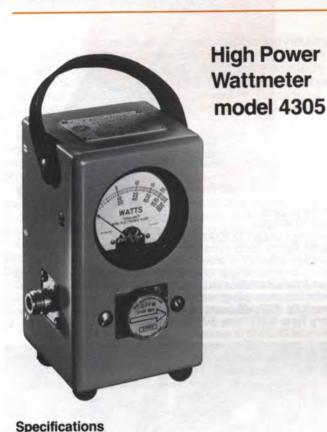
model 4305 Power Range 50W to 25000W using Bird Plug-in Elements Frequency Range 0.45 to 1800MHz Insertion VSWR with N Connectors 1.05 max. Accuracy ±5% of full scale Connectors QC Type (Female N normally supplied) Finish Light Navy grey baked enamel (MIL-E-15090) Nominal Size incl. conn. 6<sup>13</sup>/<sub>16</sub>" x 5" x 4<sup>3</sup>/<sub>32</sub>" (173 x 127 x 109mm) Weight 3<sup>1</sup>/<sub>4</sub> lbs. (1.5kg)
