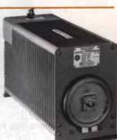
Tenuline® Attenuator Power Range 500W continuous Frequency Range & VSWR Input 1.1 max. dc to 500MHz Attenuation 30dB Accuracy ±0.5dB (±0.2dB at 30, 100, 200, 300 400 and 500MHz when using calibration data) Ambient Temperature Range -40°C to +45°C Connectors QC Type (Female N normally supplied) Coolant 0.9 gal. (3.4 liters) Refined mineral oil Operating Position Horizontal only Finish Light Navy grey baked enamel (MIL-E-15090) Nominal Size incl. conn. 171/2" x 81/2" x 515/16" (445 x 216 x 151mm)
