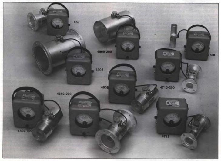
Series 4700, 4600 & 4800, 4900 Specifications: Accuracy: ±5% of full scale Insertion VSWR: 1.05 max. Finish Line Section—Silverplated, Meter Housing—Light Navy grey baked enamel (MIL-E-15090) Nominal Size Meter Housing 5%s" x 6½" x 3%" (141 x 165 x 85mm) Weight Meter 5 lbs. (2.3kg)
