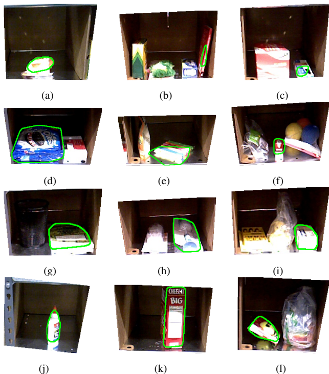
Fig. 3. Segmentation results during the APC run; the green line outlines the segments returned by our method; all segments lie on the correct objects; mean precision: 91%, mean recall: 73%, F_{0.5} score: 0.864
