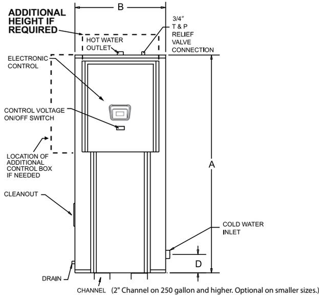
\*An oversized control panel may be required on models with inputs above 72 kW. Consult the factory for details.
