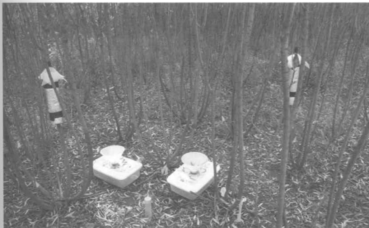
Fig. 6.31. Three-year-old willow trial on the Solvay wastebeds where sapflow, throughfall, soil moisture and various plant characteristics are being measured as part of the effort to develop an alternative vegetative cover for the wastebeds. Photo courtesy of T. Volk.
