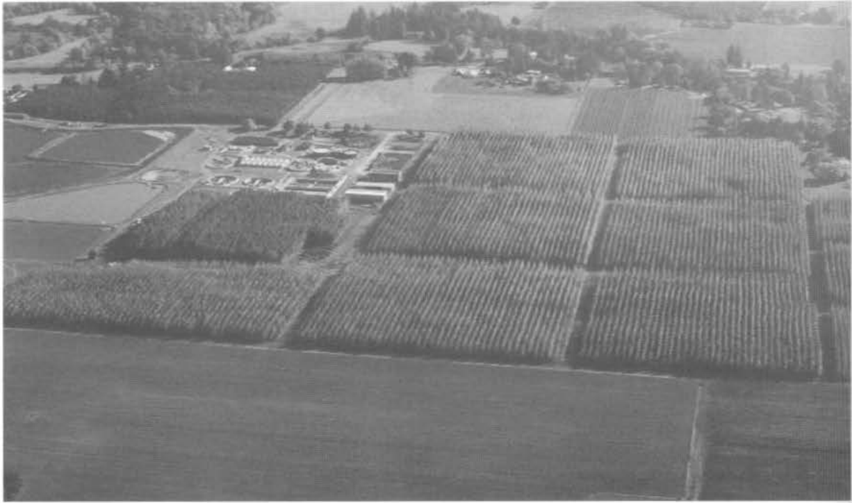
Fig. 6.32. Aerial view of the City of Woodburn, Oregon, USA, hybrid poplar stands used for treating municipal wastewater. Photo courtesy of J. Johnson.
