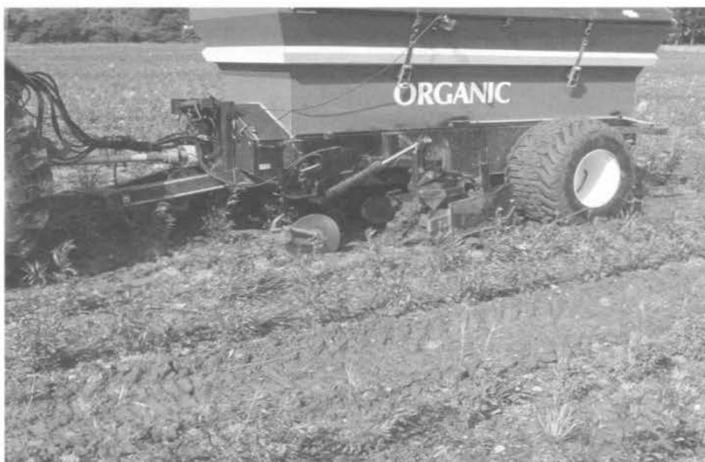
Fig. 6.28. Biosolids injection into freshly coppiced SRC willow. Photo courtesy of Rural Generation Ltd.
