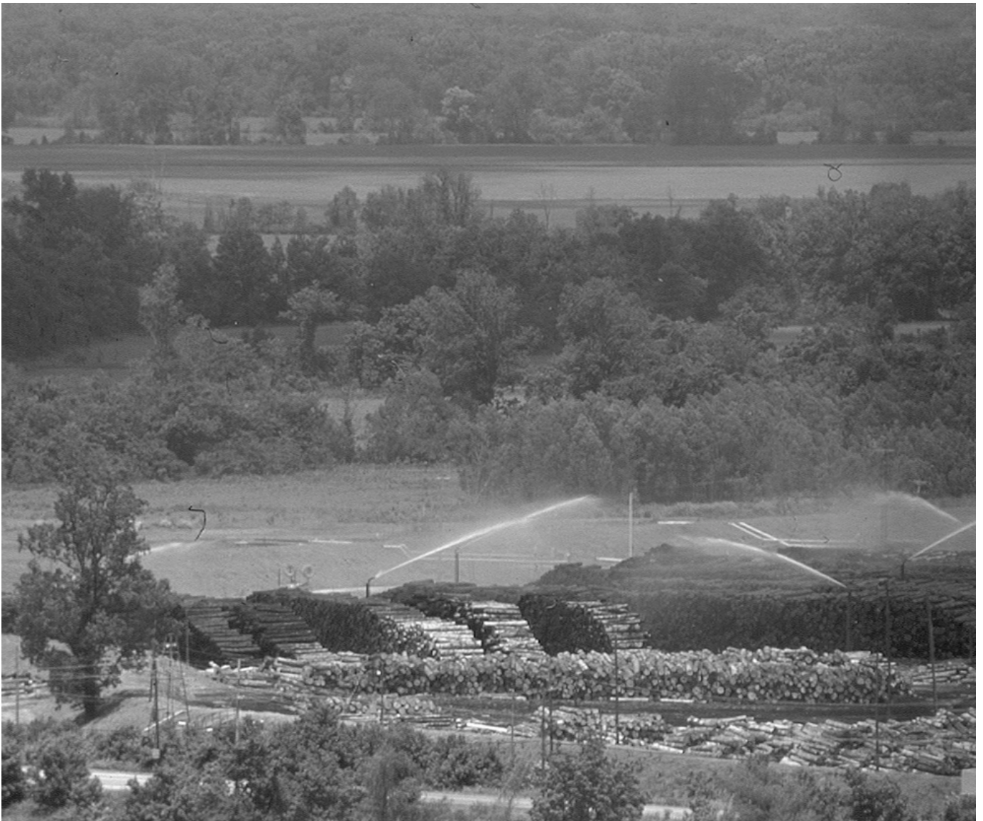
Logs are kept wet at the woodyard, Mississippi. Photo by Bill Lea
