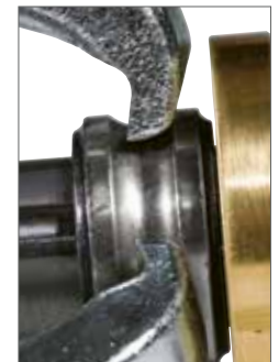
Lock on ball grooves and bearing races.
