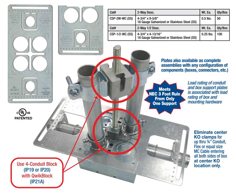
For all types of raceways installed per NEC. Accepts 4 or  $4^{11}/_{16}$  & 5" inch square shallow or deep boxes. If shallow  $(1^{1}/_{2})$  inch deep) Maximum size =  $\frac{3}{4}$  inch conduit or equal size flexible conduit or MC Cable entering box. Suitable for 1/4, 3/8 or 1/2 inch rod for support.
