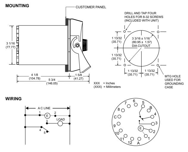
Standard CW Dial References the operation of the load when connected to terminal number 3 "ON Time" adjustment 5% to 100%
