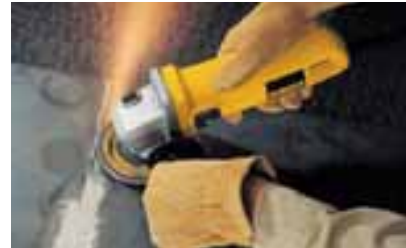
Metal fabricators use flap disks for all types of metal finishing, deburring, edge blending, chamfering and surface preparation.
