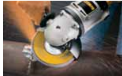
Welders use flap discs for weld blending, removing weld slag, deburring surface finishing and chamfering.
