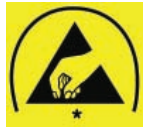
Symbol for packaging materials * primary code L = Low Charging, C = Conductive, D = Dissipative, S = Shielding
