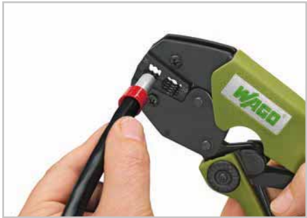
Insert ferruled conductor into crimping station.
