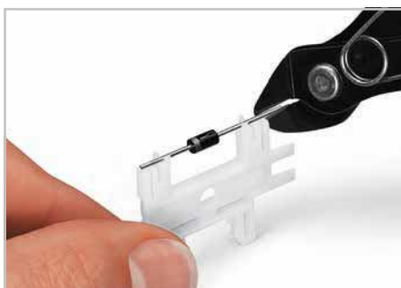
Cutting component to the proper length.
