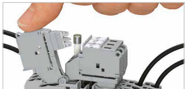
Pivoting the fuse holder open to the locked position. Fuse terminal blocks for miniature metric fuses rated at 2.5 mm 2 (12 AWG) and 6 mm 2 (8 AWG)
