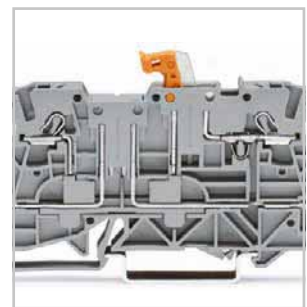
Variant: One disconnect and one through terminal block are accommodated on two levels in a terminal block that is just 5.2 mm wide.
