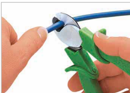
Cutting a conductor.
