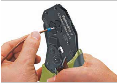
Insert ferruled conductor into crimping station.
