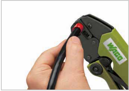
Squeeze handles until ratchet mechanism is released.
