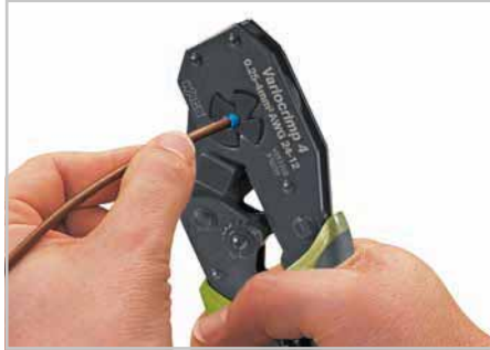
Squeeze handles until ratchet mechanism is released.
